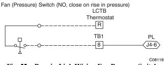
Fig. 55 - PremierLink Wiring Fan Pressure Switch Connection
